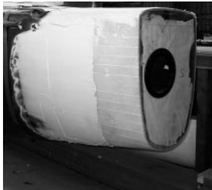
(left) The stern has been lengthened with corecell strips. (right) The bow has side shins over temporary molds. The starboard bow is complete, but for a 1' nose.
