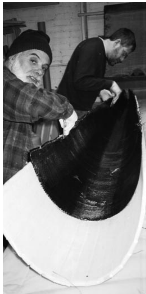
Ted Warren (front) and Ted Grossbart (rear) laying up the inner carbon skin of the new bow section prior to vacuum bagging.
