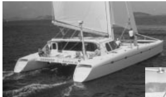
Designed for a serious ocean sailor, Bill Matthews, Shearwater featured lift up rudders and folding props for easy navigation in shallow water. The well-appointed bridgedeck (right) would please any sailor's wife.
