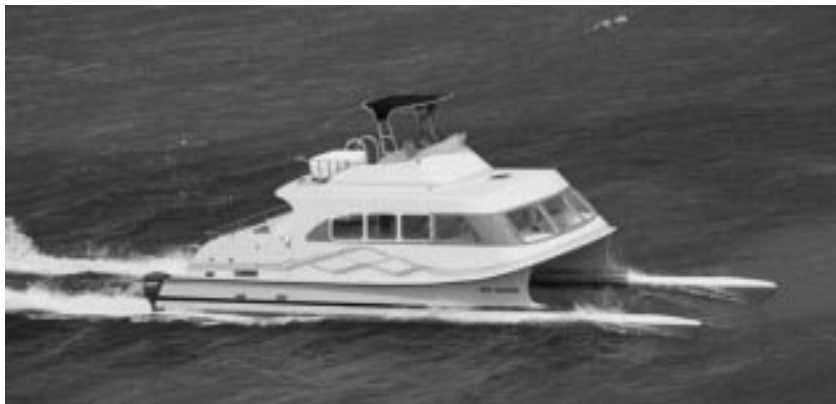
Wave piercer commercial motor catamaran pierces through the waves rather than over them, which according to Jim Brown, results in the "smoothest ride for the best speed and the least cost".
