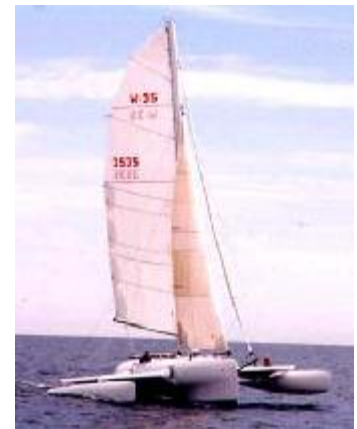
1997 Warren 35 trailerable trimaran, "Veloce". Custom designed for fast coastal cruising/comfortable racing. Spacious interior with over 6 foot headroom and large berths. Enclosed head with holding tank. Built by Maine Cat using fiberglass over Core-Cell foam. Composite Engineering carbon fiber beams and wing mast. Main, self-tacking jib, screecher. 9.9hp four-stroke Yamaha. Custom trailer. $125,000. Located in Beverly MA. Steve Mclafferty mclafferty@alum.wpi.edu or 781-405-1234.
