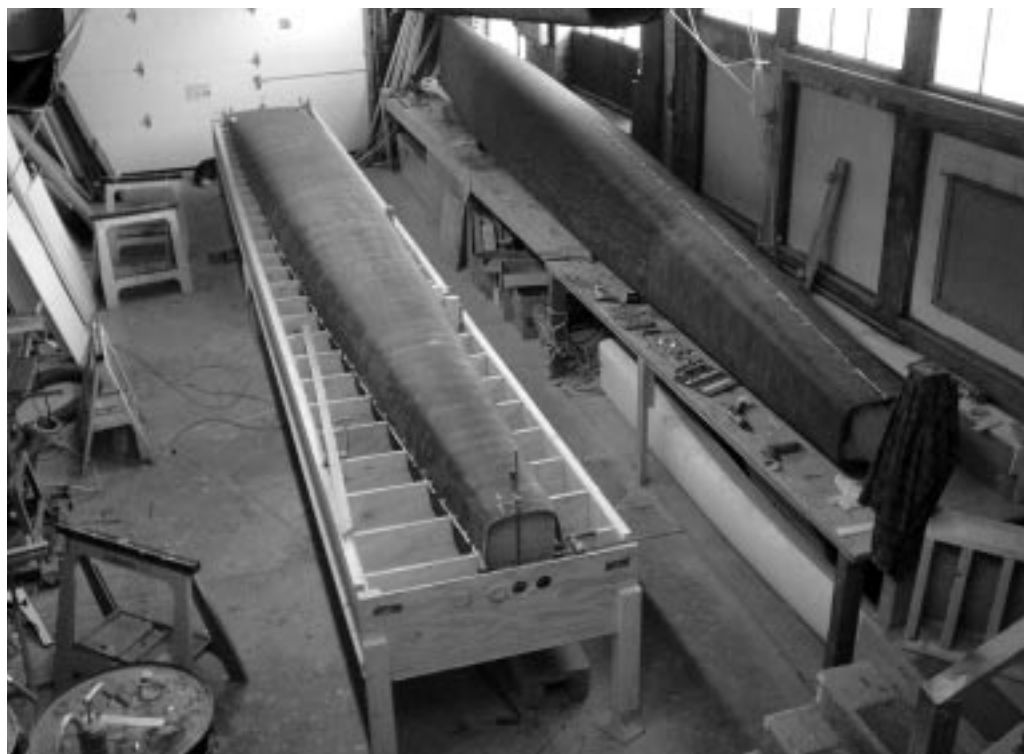
Ariel view of a half-ama lying on the strong back (center). A complete ama lies on the workbench (right).
