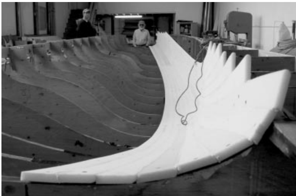
Core-Cell planking is laid into a half-hull mold built of plywood stations bolted to a strong back. Note the cove and bead joints between "planks".
