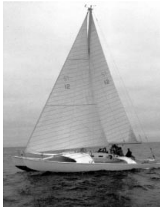
Moxie , Newick-designed 50' trimaran in which Phil Weld won the 1980 single handed transatlantic race. Note original low aspect rig. Cover photo shows new fractional rig.
